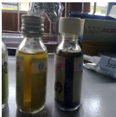
Figure 4 Water sample showing positive result for H 2 S test (black colour)
