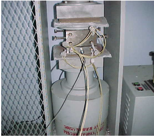
Figure 3 Mould of Hip prosthesis along with heating arrangement placed in compression machine
