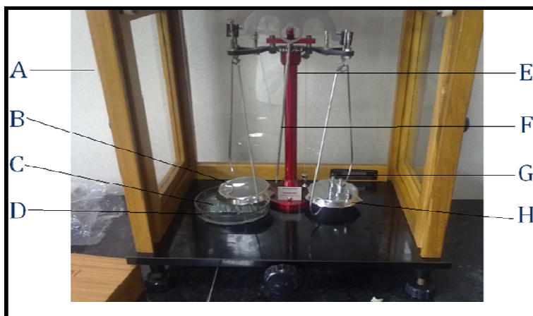
Figure 3 In-vitro mucoadhesive strength measurement apparatus.
