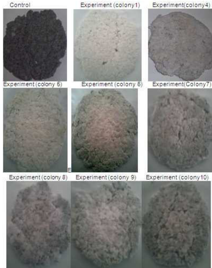
Figure 4 Manually pressed pulp before and after treatment with bacterial culture
