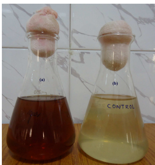
Figure. 1 Silver nanoparticles synthesized by Ulva lactuca in an aqueous solution of silver nitrate (a) with control (b)
