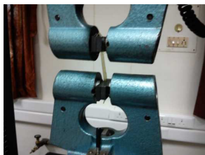
Figure 4 Position of hydrogel sheet during tensile strength testing
