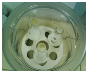
Figure 2 shows the water vapour transmission test method
