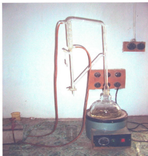
Figure 4 Clevenger's Apparatus used for extraction of essential oil
