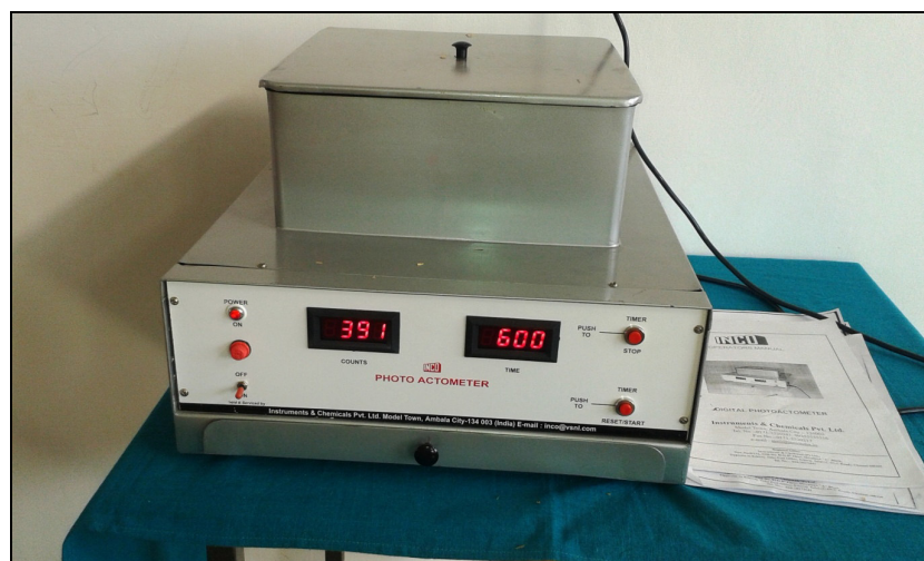
Figure 1 Locomotor activity by using Digital photoactometer in experimental model (control group-saline treated)
