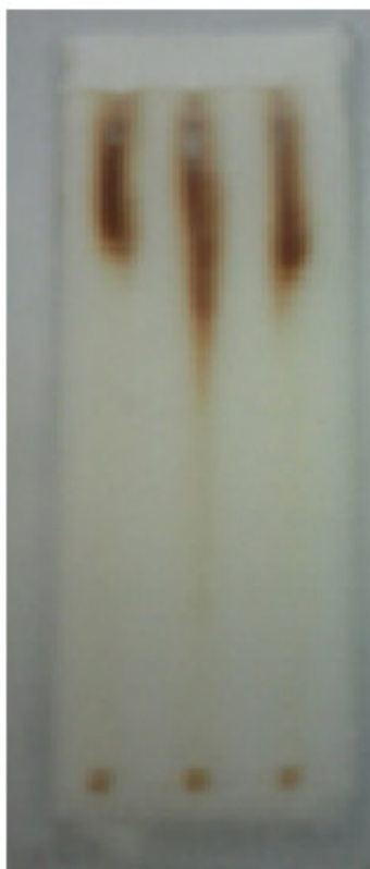
Figure 1 Separation of alkaloids from the solvent extract of dried leaf powder from Catharanthus roseus using thin layer chromatography
