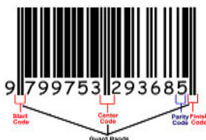
Figure 1 Example of 1D barcode (EAN13 barcode)
