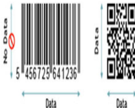
Figure 2 Example of ID Barcode and 2D Barcode (QR CODE).
