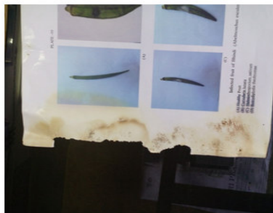
Figure 2A Paper infested by cellulolytic fungi (Source of the test fungus – Curvularia lunata )
