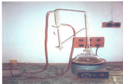
Figure 4 Clevenger Apparatus for extracting essential oils
