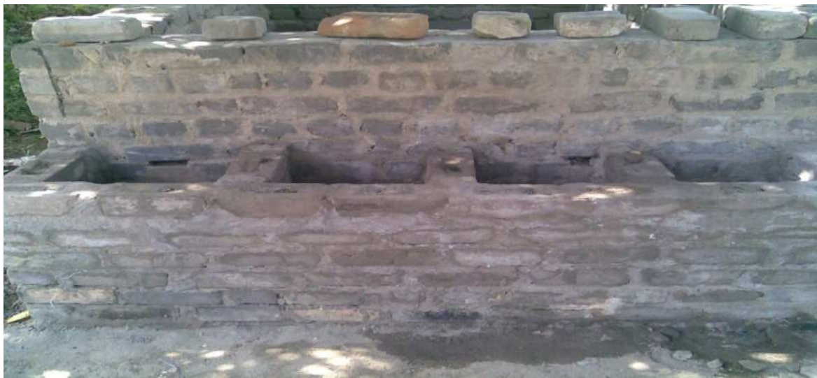
Figure 1 Compost pits in order A(80:20),B(60:40),C(80:20)+nutrients and D(60:40)+nutrients FIELD TRIALS
