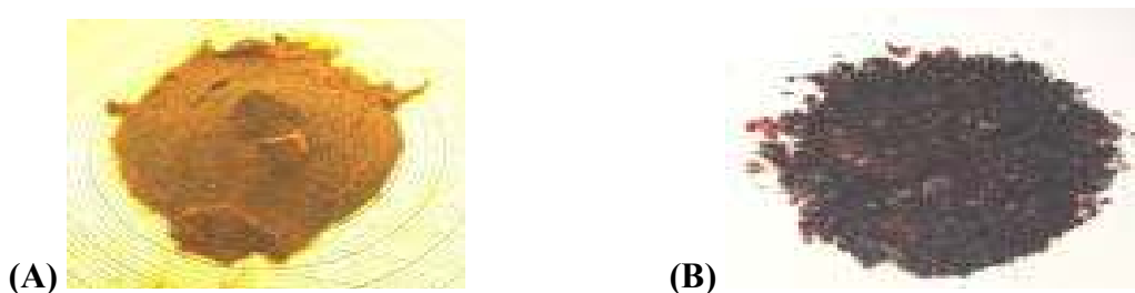
Figure 1.1. Freeze-dried aqueous extract of Corchorus olitorious leaves (A) and hygroscopic nature of powder after exposure to high humidity (B)
