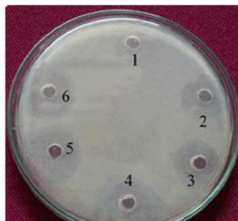
Fig 1 Antibacterial activity of ZnO nanoparticles against S. aureus (Kirby-Bauer test)
