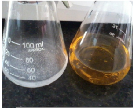
Figure:2 Synthesis of silver nanoparticles by chemical method
