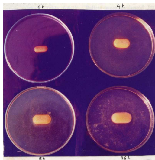
Figure 3 Photograph of tablet L 4 during in-vitro dissolution studies at 0 h, 4h, 8h and 16 h time period
